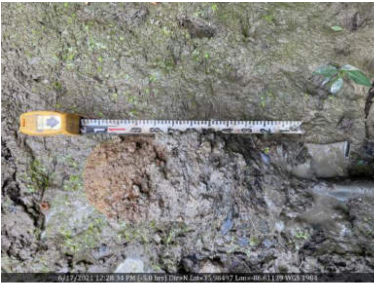
28 View of ISOPND-A soil profile with clay liner starting at approximately 7 inches, facing down.
