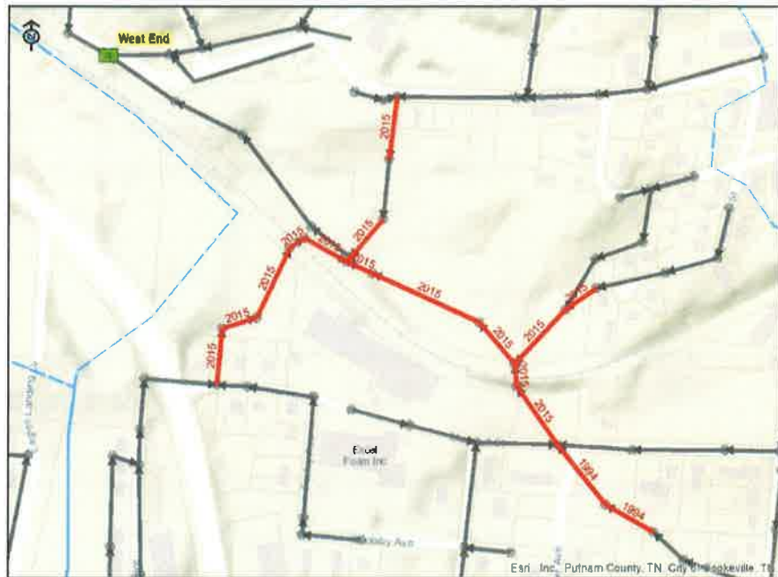
Figure 5, Lines with CIPP installed
