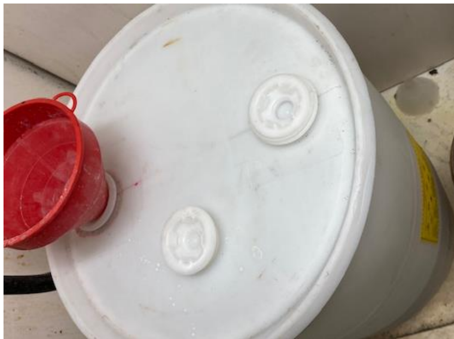
Photo 35, 30-gallon hazardous waste accumulation container, hazard indication is corrected vs. the June 9 initial inspection, but the container was found open, Buehler 665, August 24
