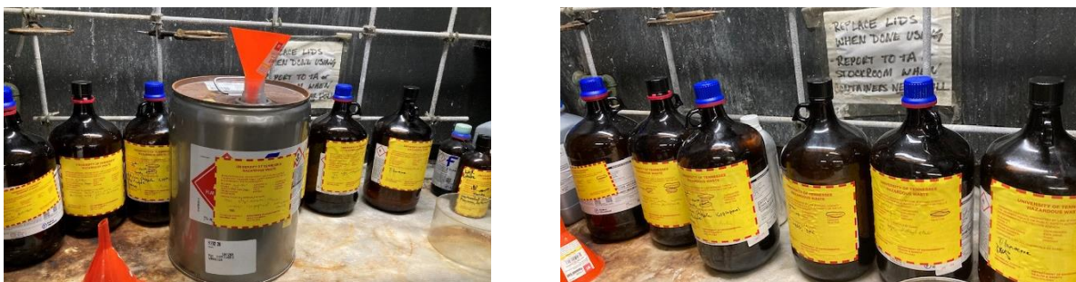
Photos 27 and 28, open container found in June, left, and same lab but with two of the lids found loose, Buehler 630, August 24
