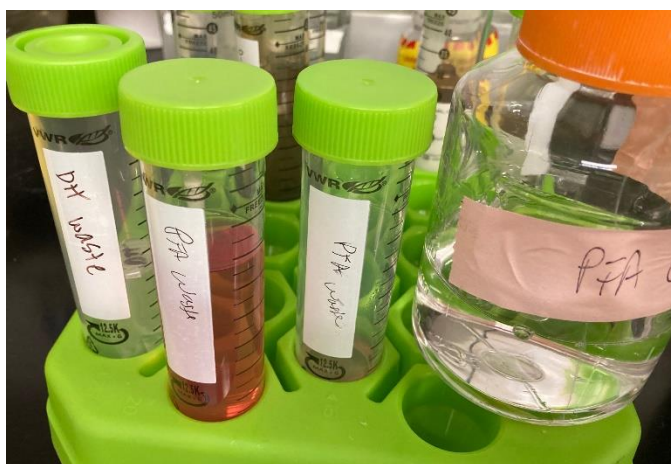
Photo 61, hazardous waste container not marked “hazardous waste” nor to indicate the hazard, Mossman 420D, August 24
