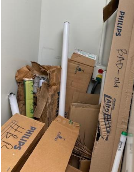
Photos 52 and 53, one open container of “bad – old” lamps (left) observed on June 8; during the follow-up inspection, this same container (right) was observed open and not properly marked on August 24. Uncontained lamps of uncertain condition are visible in both photos. Hesler Hall 126, August 24.
