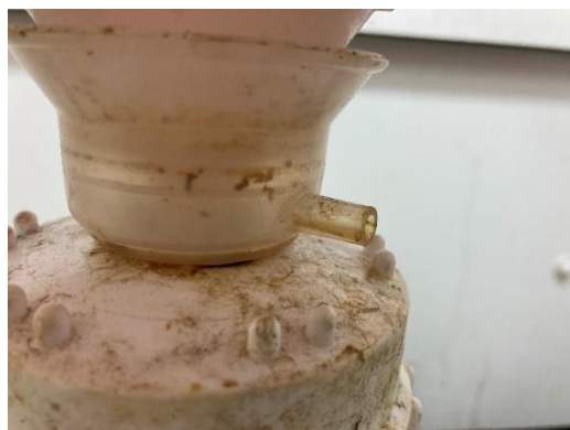
Photos 65 and 66, hazardous waste containers in the general chemistry labs showing the detail of the vent-port (left) and the three-bottle accumulation setup (right) with the vent-ports attached, Strong Hall general chemistry labs, June 9
