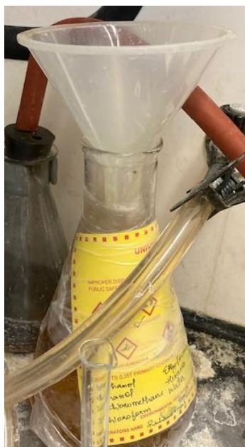
Photos 36 and 37, open hazardous waste satellite accumulation containers under hood numbers one (left) and four (right), Buehler 665, August 24
