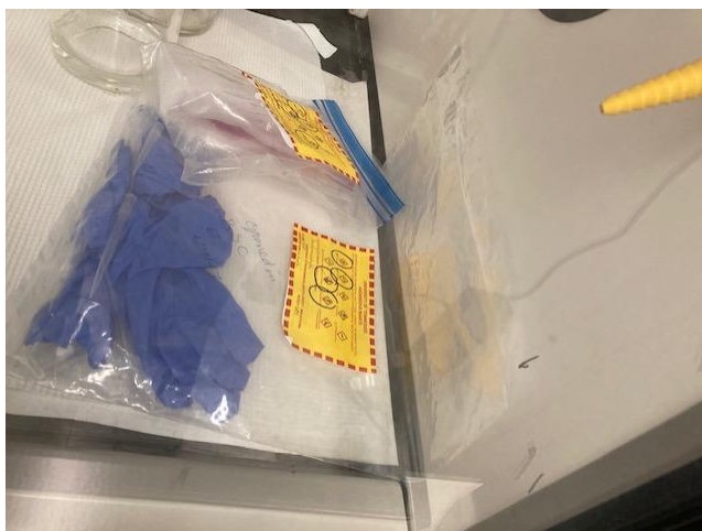
Photo 11, plastic bags containing hazardous waste, both closed and marked, SERF 604, August 24
