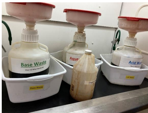
Photos 65 and 66, hazardous waste containers in the general chemistry labs showing the detail of the vent-port (left) and the three-bottle accumulation setup (right) with the vent-ports attached, Strong Hall general chemistry labs, June 9
