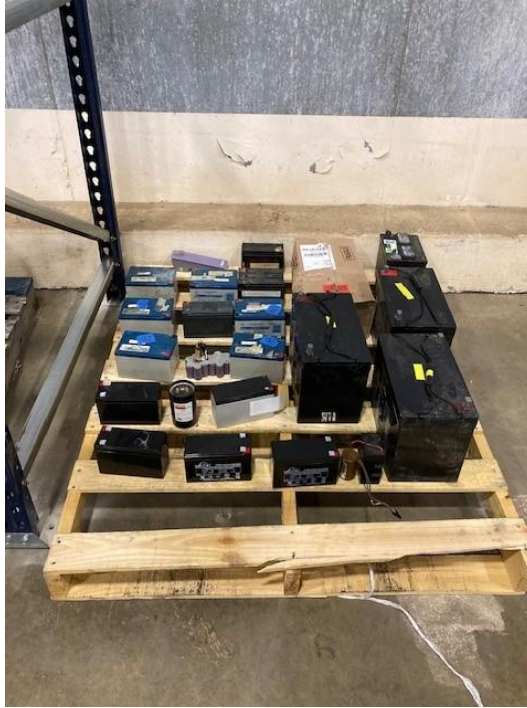
Photo 9) At the Fleming Center, facility staff failed to place storage dates and universal labeling on each lead-acid waste battery on the pallet.
