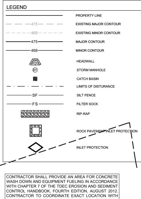
CONTRACTOR TO COORDINATE EXACT LOCATION WITH NPDES DEPARTMENT DURING PRECONSTRUCTION MEETING. CONTROL OF OTHER SITE WASTES SUCH AS DISCARDED BUILDING MATERIALS, CHEMICALS, LITTER, AND SANITARY WASTES THAT MAY CAUSE ADVERSE IMPACTS TO WATER QUALITY IS ALSO REQUIRED BY THE GRADING PERMITTEE.
