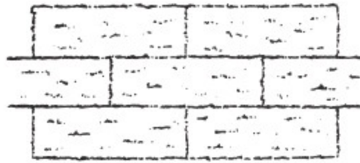
Figure 7-7.10-1. Correct sod placement
