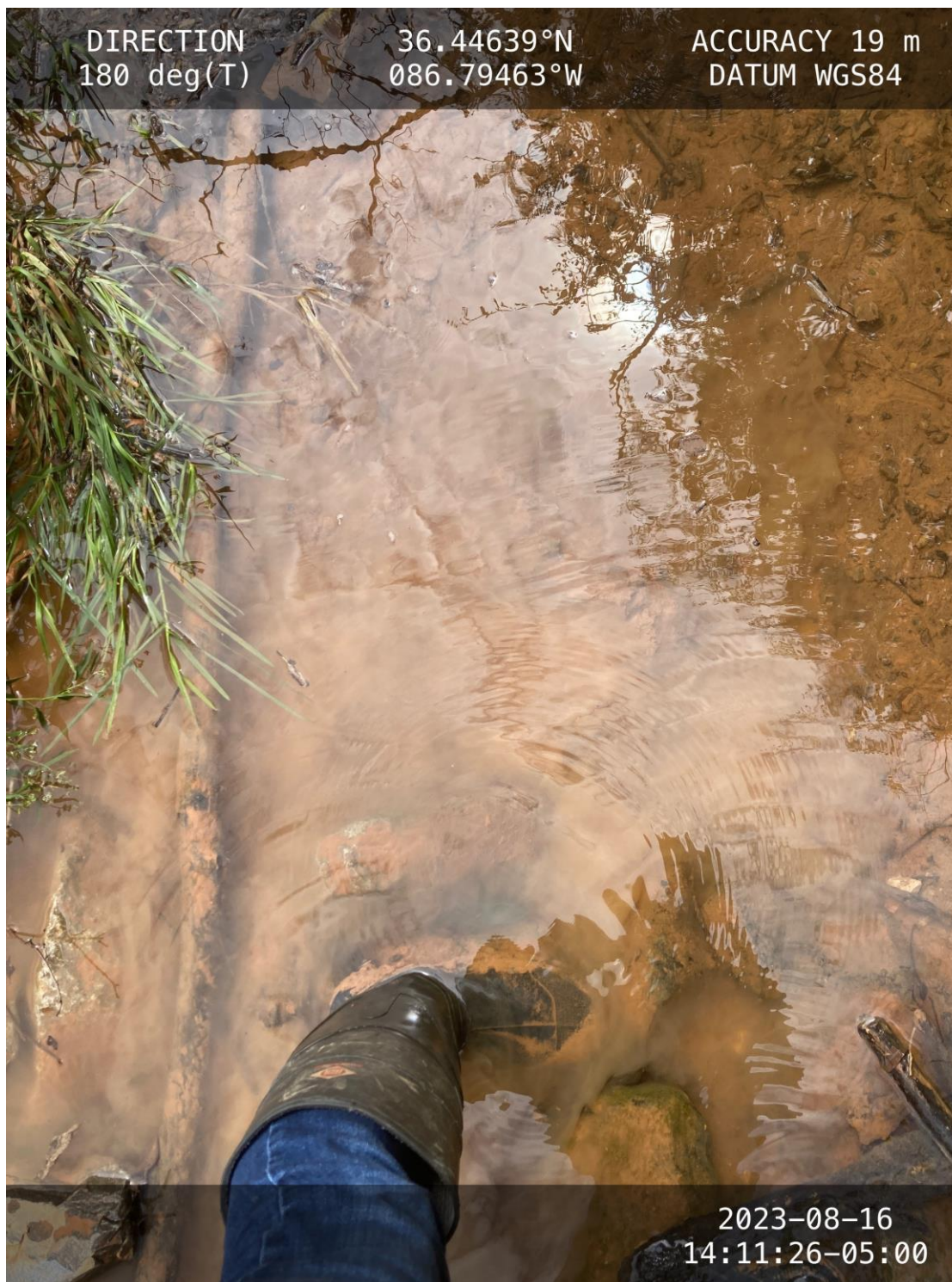
Attachment 3: sediment deposition approximately 4 inches at outfall
