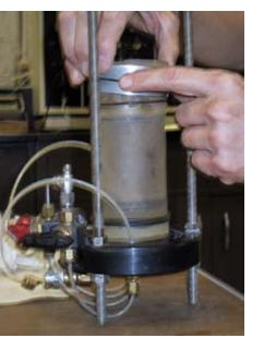
Preparing sample in cell for flexible wall permeability test
