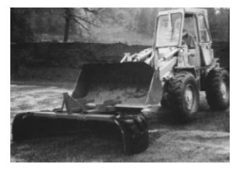
Figure 12–12 Lawn and garden tractor scraping equipment (courtesy Kubota Tractor Corporation)
