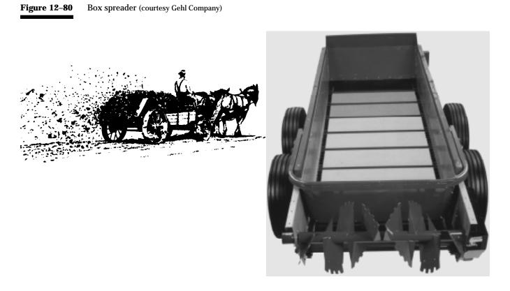
The load capacity of tractor-tow and truck-mounted box spreader models ranges from about 20 to more than 400 cubic feet. The ASAE Standard S324.1, Volumetric Capacity of Box Type Manure Spreaders (ASAE [f] 1990), is used by manufacturers to provide uniform load capacity ratings (in cubic feet) of different box spreader models. Some advertising materials, however, use bushels, gallons, or tons. See Conversion Factors and Tables of this handbook.
