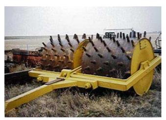
Figure 10D–19 Modern type of tamping roller less well suited for compacting soils for clay liner
