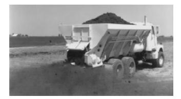
A hydraulic-lift dump box truck designed to haul gravel and grain is also useful to haul feedyard poultry litter and other solid waste (fig. 12–86). These alternative uses should be considered in selecting hauling and spreading equipment. The dump box capacity typically ranges from 4 to 12 cubic yards. Actual weight or volume of waste hauled depends on the waste characteristics and the dump box design. Spillage problems are minimized if the load is correctly trimmed, wetted down, or covered.
