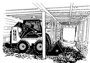
Overall height and width clearances are important for maneuverability. A loader bucket width, the same or wider than the tractor width, aids steering when scraping; and reduces tracking spilled waste. Buckets range from 3 to 6 feet wide.
