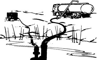
The practical limit of liquid suction for most centrifugal pumps is 22 feet at sea level, 17 feet at 5,000-foot elevation, and 14 feet at 10,000-foot elevation. Pumps will operate beyond these limits, but their performance is seriously reduced by cavitation or nonuniform liquid flow through the pump. Elevation can also affect vacuum pump suction and pumping performance (see fig. 12–88).
