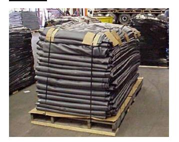
wooden pallets) and stacked no more than two to three rolls high, as shown in figure 10E–2. Panels of material should be shipped and stored on a pallet, as shown in figure 10E–3, and should not be stacked unless contained within a crate.
