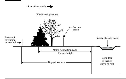
Figure 8–27 Fences affect snow and soil deposition around buildings.
