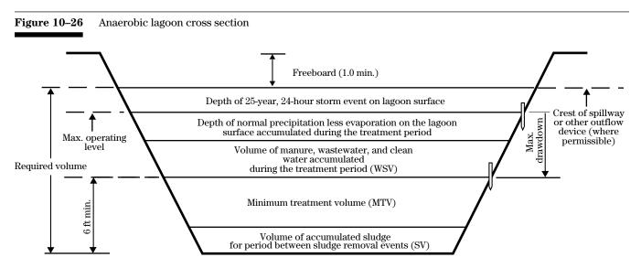
Note: The minimum treatment volume for an anaerobic waste treatment lagoon is based on volatile solids.
