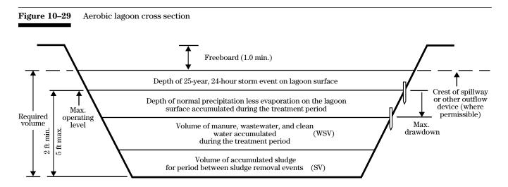
Note: An aerobic waste treatment lagoon has a required minimum surface area based on BOD5
