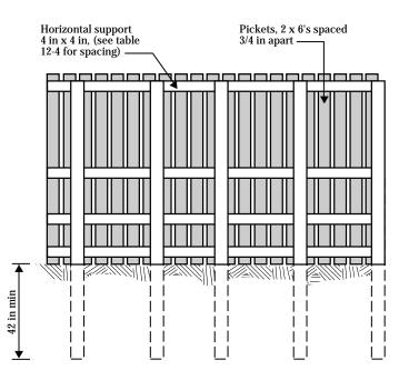
Picket dams are designed to allow runoff from the pile surface at any height within the range allowed by the stacking facility. The dam utilizes vertical slots because they drain and clean better than horizontal slots. The picket dam is located so that a clear drainage path is always away from the face (leading edge) of the pile. Drainage water that exits the dam is collected and transferred to a liquid waste storage facility. Table 12–4 gives construction information for picket dams.
