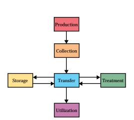
The waste management system should identify the storage period; the required storage volume; the type, estimated size, location, and installation cost of the storage facility; the management cost of the storage process; and the impact of the storage on the consistency of the waste.
