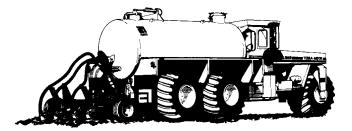
Uniform spreading by gravity flow out of a tanker is difficult. The solids can partly block the tank discharge or less waste will flow as the waste depth in the tank decreases. Also, as the load lessens, travelspeed changes. European engineers have developed an electronic flow control interlocked with a groundspeed monitor (fig. 12–91) that automatically adjusts tanker unload flow according to a preset outlet valve pressure (Carlson 1991, Malzeryd 1991).
