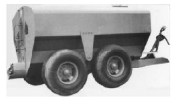
Figure 12-83Flail type side unload spreader (Bartok<br/>1994) (courtesy Ideal Industries Inc.)
