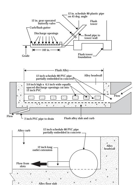
holes had a 1-foot-long outlet extension and allowed flushwater volume to uniformly, but forcefully, exit into the alley as seven smaller streams rather than a large, concentrated stream. In daily flushing, the cleaning done by the spaced-hole flushwater discharge was preferable to the dump type flushtanks and the air-controlled pipe valve flushwater dischargers (Patrico 1992).
