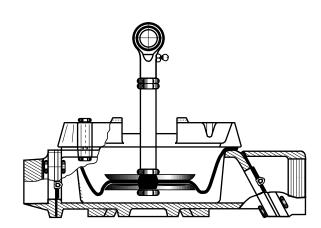
The diaphragm pump is commonly use by custom operators that pump or haul sewage sludge where performance is more important than high capacity. It is also used as a hand-operated primer pump with a high capacity centrifugal pump. Another common use for this type pump is for an automobile fuel pump. It can operate dry and be relatively trouble free with liquid and slurry wastes.
