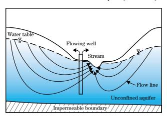
Figure 7–7 Cross section through stream valley showing groundwater flow lines and flowing (artesian) well from unconfined aquifer (Fetter 1980)
