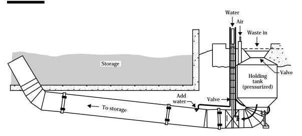
Although the investment for this type of equipment is relatively high, operating cost is low. Solid waste and freezing can restrict flow, and sand and excess soil in the waste can settle out and buildup in the pipe that leads to the storage tank.
