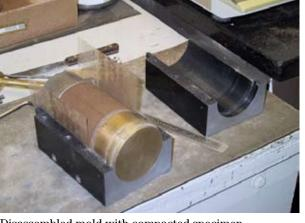
Disassembled mold with compacted specimen
