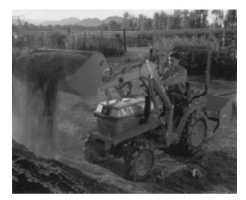
capacity, the tractor framework, traction, and overturning are limitations. Elements to consider in selecting a loader are the operator's view, quick attachment, clearances, operating speed, and joystick type hydraulic control.
