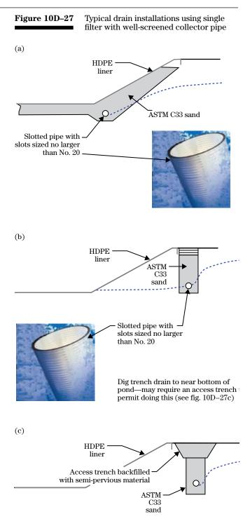
Illustrated access trench construction to permit installing deeper trench drain. Access trench filled with semi-pervious soil to limit infiltration of surface runoff.
