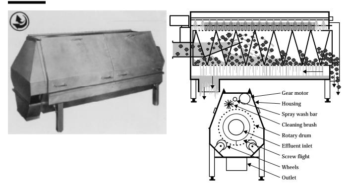
electric motor is used for throughput of 10 to more than 5,000 gallons per minute, depending on the waste type. A separated solids portion to about 30 percent dry material is possible.
