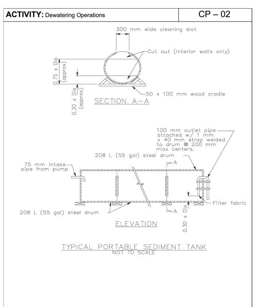
CONTRACTOR SHALL BE RESPONSIBLE FOR DEWATERING OF EXCAVATION DURING THE CONSTRUCTION PERIOD IN ACCORDANCE WITH SECTION CP-02 OF THE NASHVILLE METRO STORMWATER MANAGEMENT MANUAL VOLUME 4. THE BOX SELECTED SHOULD BE MADE OF STEEL, STURDY WOOD
