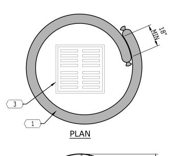
**KEYNOTES** DESCRIPTION | SILTATION EEL DEVICE (SOCK); USED IN AREAS WHERE EXISTING PAVEMENT PREVENTS THE USE OF SILT FENCE; STABILIZE THE SILTATION EEL BY PLACING SANDBAGS AS NEEDED ON TOP OF THE 2 | PAVEMENT SURFACE 3 INLET STRUCTURE GRATE
