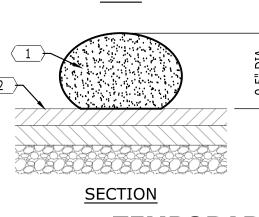
**TEMPORARY SILTATION EEL INLET PROTECTION (TCP-24)** NOT TO SCALE
